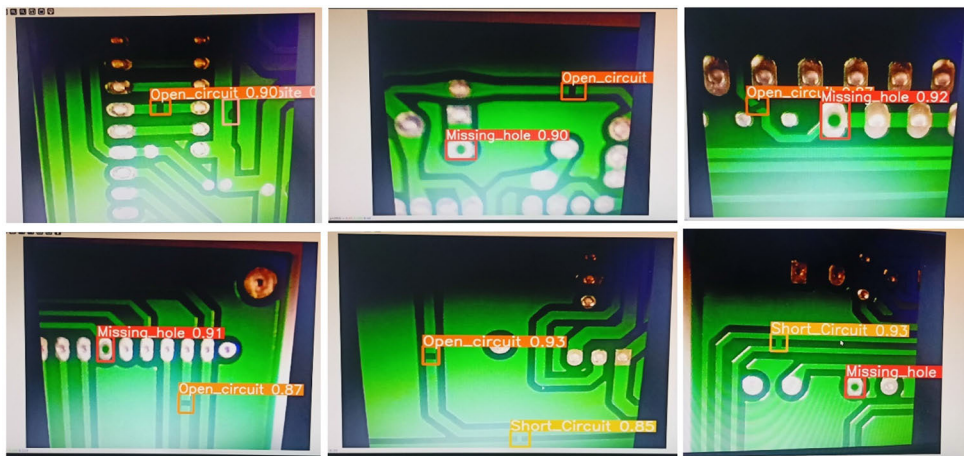
FIGURE 10. Performance of the real-time PCB defect detection system using the MDD_PCB dataset.
