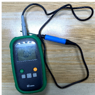
FIGURE 15. Finger Tesla meter.
