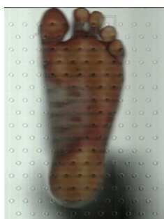
FIGURE 5. Scanned plantar surface image example through perforated sheet.
