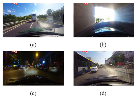
FIGURE 1. Depiction of complex driving conditions for lane analysis: (a) Curvature handling improvements via Angle Loss, (b) Semantic dependence during intense lighting, (c) Situations lacking clear lane markings, (d) Obstructions from vehicles in lane visibility.
