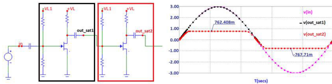
FIGURE 68. Characteristics of a stage: a) Limiting circuit & b) Saturated sinusoidal signal.
