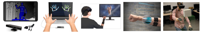
FIGURE 5. Different ways of tracking motion in AR. From left to right: Kinect® camera, Leap Motion®, inertial 7DOF motion sensor, Myo® and Hololens® controller.
