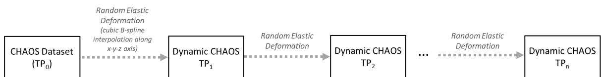
FIGURE 2. Flowchart of dynamic data generation. In this work, n = 24 and the total number of TP is 25 timepoints.
