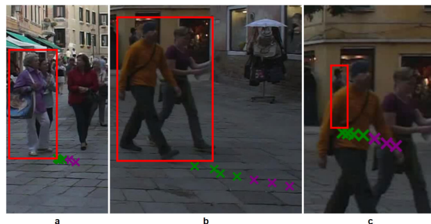
FIGURE 8. Pedestrian group trajectory prediction on a sample frame of the MOT17 dataset.
