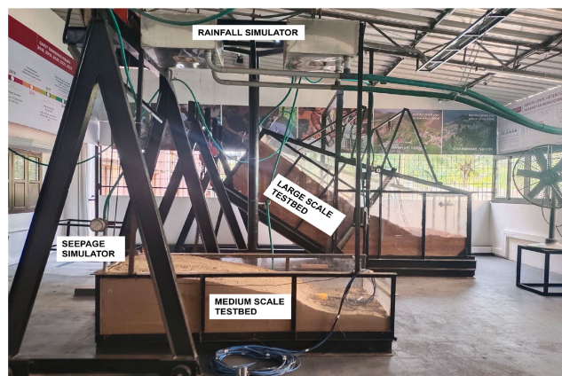
FIGURE 4. Set up of landslide testbeds.
