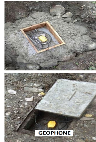
FIGURE 6. Geophone sensor placement at the deployment site at Chandmari, Sikkim.
