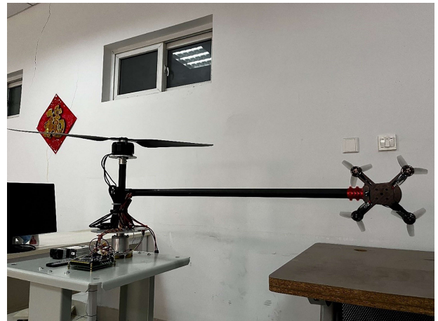
FIGURE 5. Overall physical image of the unmanned helicopter distributed electric tail rotor test stand.
