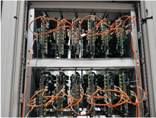
FIGURE 5. Prototype of fiber optic networking dynamic mode equipment, where 54 SCE boards are adopted as sub-modules for networking. By using few physical sub-modules can achieve full access testing of large-scale node valve control, thereby reducing the cost of power testing for the key equipment in the power system, e.g., driver boards, high-voltage power supplies.
