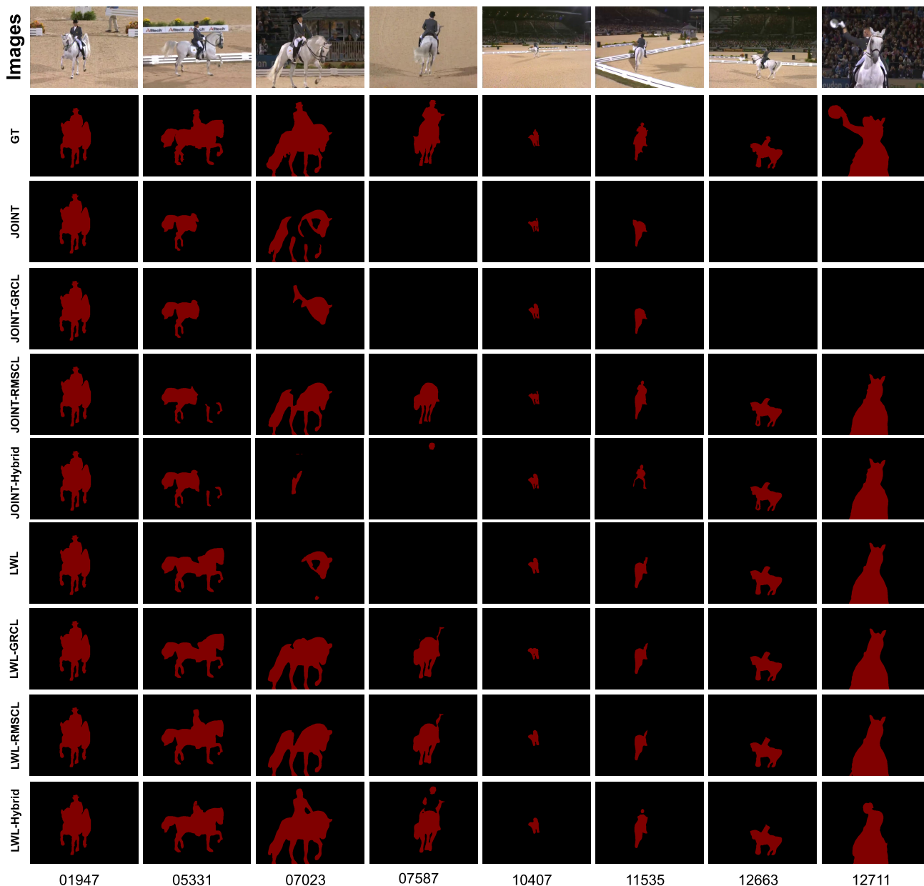
FIGURE 6. Qualitative comparison of the competing frameworks in the context of the long-video dataset. The associated frame number for each image is shown along the bottom. The leftmost column shows the given mask Y_g , which is the same for all methods. The results show that the proposed GRCL, when augmenting the baseline frameworks (LWL and JOINT), can lead to better performance against representation drift. Additionally, the frameworks based on RMSCL (LWL-RMSCL, JOINT-RMSCL) are less vulnerable to the distribution changes which take place in long video sequences. LWL-Hybrid clearly has the best performance among the compared methods.
