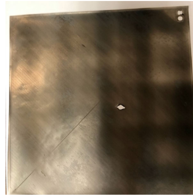
FIGURE 4. The 80 \mu\text{m} sample after the puncture occurred.
