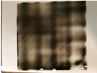
FIGURE 1. 60 \mu\text{m} thickness plate with obvious flaws.
