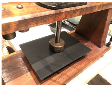
FIGURE 3. Test setup showing the DUT (ABS plate).
