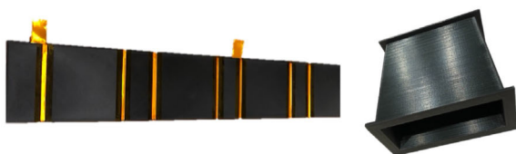
FIGURE 7. 3D printed ABS bobbin and insulation between inductor’s turns.
