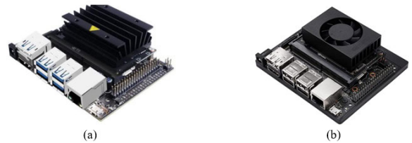
FIGURE 11. (a) NVIDIA Jetson Nano 4GB Developer Kit B01 (b) NVIDIA Jetson Xavier NX Developer Kit.
