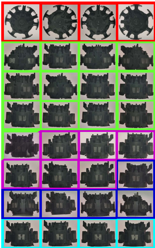
FIGURE 8. The defects on physical parts coincide with the clustering of the associated production parameters in the latent space of the autoencoder, highlighted with the same colors in Fig. 7.
