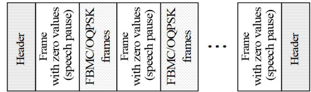
FIGURE 4. Structure of the speech-like FBMC/OQPSK signal.
