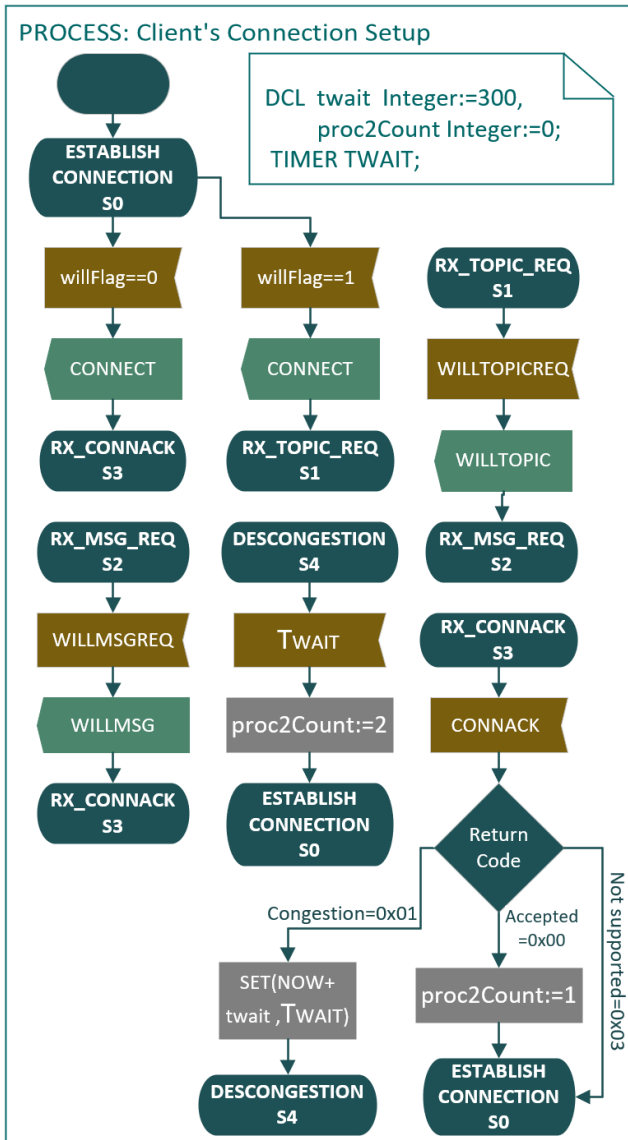
FIGURE 21. SDL process for the client, representing the configuration for the client connection.
