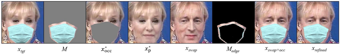
FIGURE 13. Face and mask images for each step of the occlusion handling framework. We extract the mask explicitly and transfer the extracted mask back onto the swapped face.
