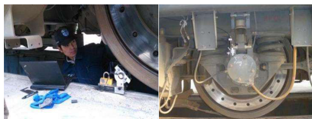
FIGURE 19. Measurement of (a) wheel polygons and (b) ABA using the MÜLLER-BBM device and accelerometer, respectively [36].
