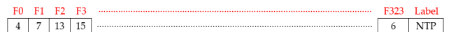
FIGURE 2. An example of one sample of DL model input that ranges from element F0 to F323 along with their decimal values and is followed by the attack label.
