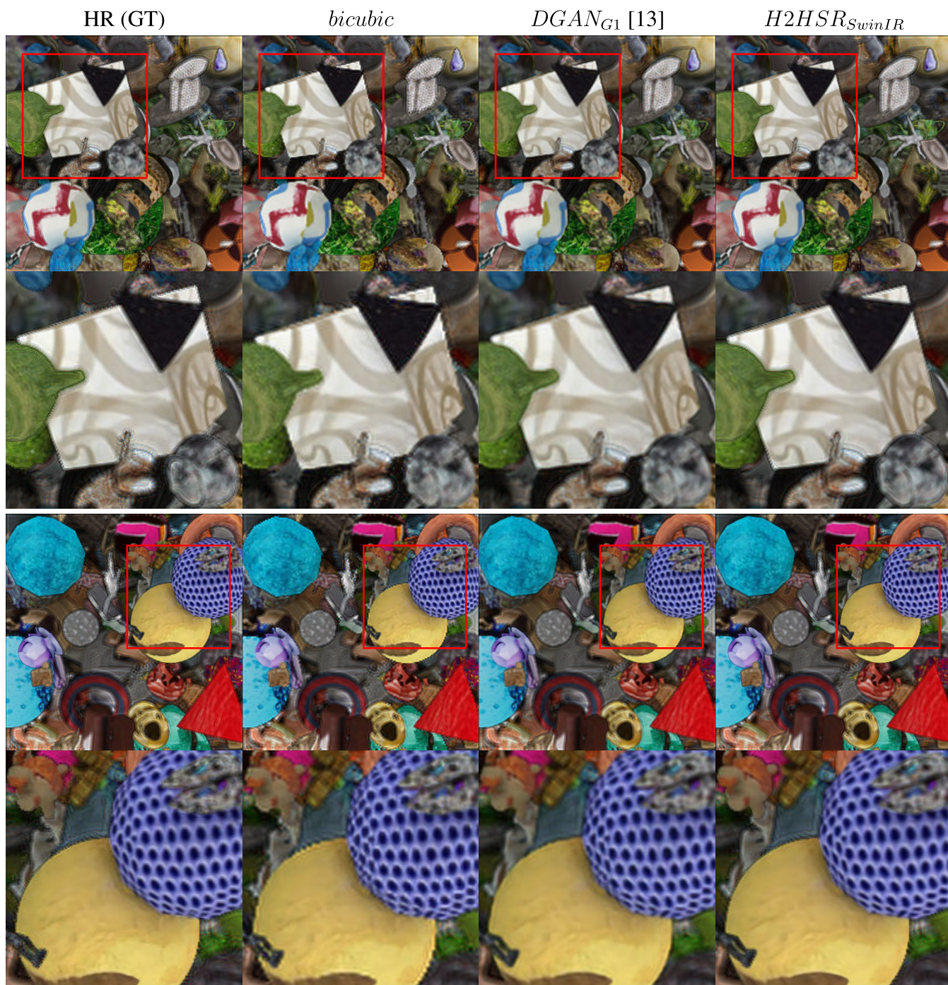
FIGURE 2. Numerical reconstruction results obtained from hologram super-resolution using three different methods. The focused objects are highlighted within red boxes, and the second row provides magnified views of these regions. More comparison results are available in the supplementary report.
