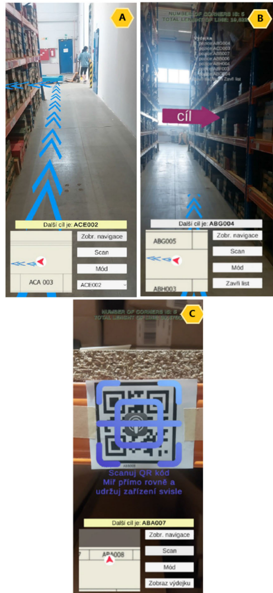
FIGURE 6. User interface: A - manual mode, B - visual target identification (CÍL means TARGET), C - marker scanning.
