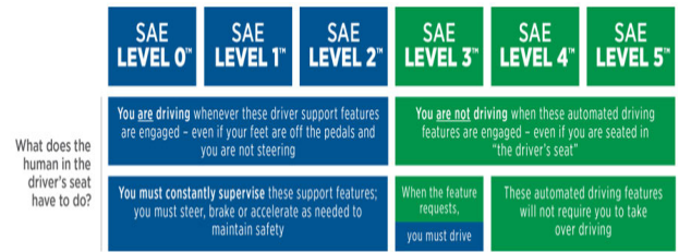
FIGURE 1. Levels of driving automation based on SAE standard [15].
