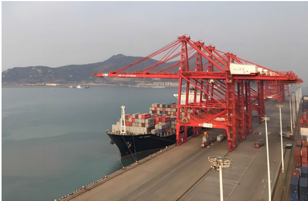
FIGURE 2. Array of discharging container cranes operating on-site, working together to load and unload containers for the same cargo ship.
