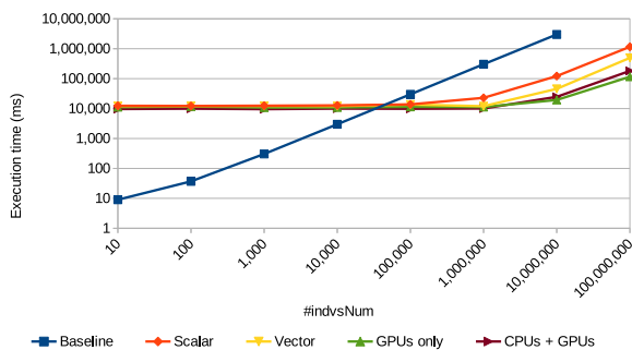
FIGURE 7. Visualizing experiment 2 results using log-log plot: the performance impact of evaluating 100,000 hypotheses on #ivsNum individuals.
