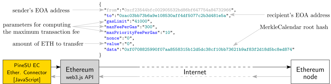
FIGURE 10. Illustration of a regular ETH transaction triggered by a registration operation of PineSU, through its Ethereum connector. All the SUs in the storage group being registered must have the same owner in their pinusu.json file, which must coincide with the sender's EOA address ( from attribute). The EOA addresses of the sender and the recipient are both controlled by the same person. The from key and its value are colored gray, since they are not explicitly included in the transaction data, but they can be obtained indirectly; namely, every transaction must be signed by the sender, who has to be identified to verify the signature.
