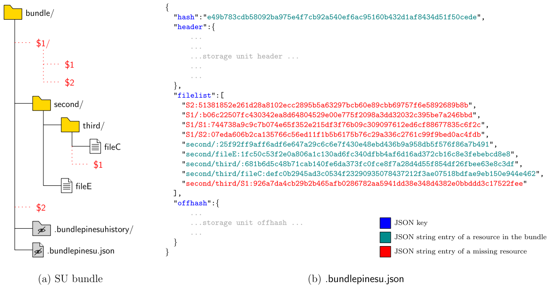
FIGURE 8. An example of a storage unit bundle. (a) Missing SU resources are represented with no icon and with a red $count placeholder. (b) Illustration of the corresponding .bundlepinesu.json hidden file included in the bundle; entries of resources in the bundle are colored in teal, whereas those of missing resources are in red.
