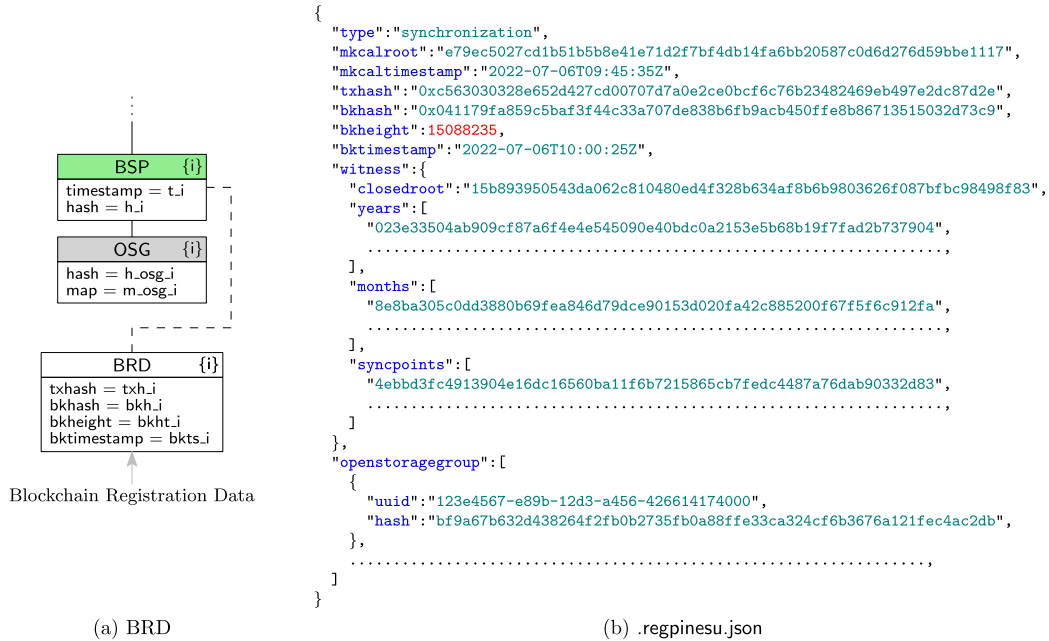
FIGURE 11. Illustration of how the blockchain registration data are stored in PineSU, in case of a synchronization operation. (a) A BRD element is associated with the corresponding BSP node in the MerkleCalendar. (b) Blockchain registration metadata for a specific SU in the synchronized OSG; the metadata are stored in the .regpinesu.json hidden file (in the root folder of the SU) which is tracked by Git.
