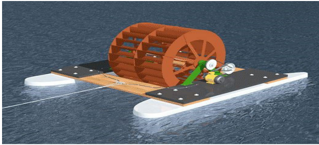
FIGURE 3. Shows the concept of floating waterwheel power generators [55].
