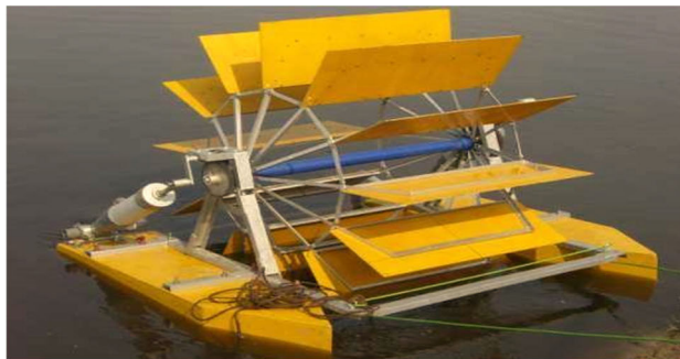
FIGURE 5. Floating power generator on site [54].
