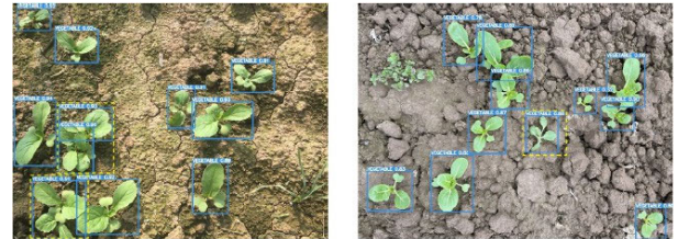
FIGURE 17. YOLO-v3 failed to cover all vegetables due to occlusion, with yellow dashed boxes representing missed detection and yellow dashed boxes representing erroneous detection [108].
