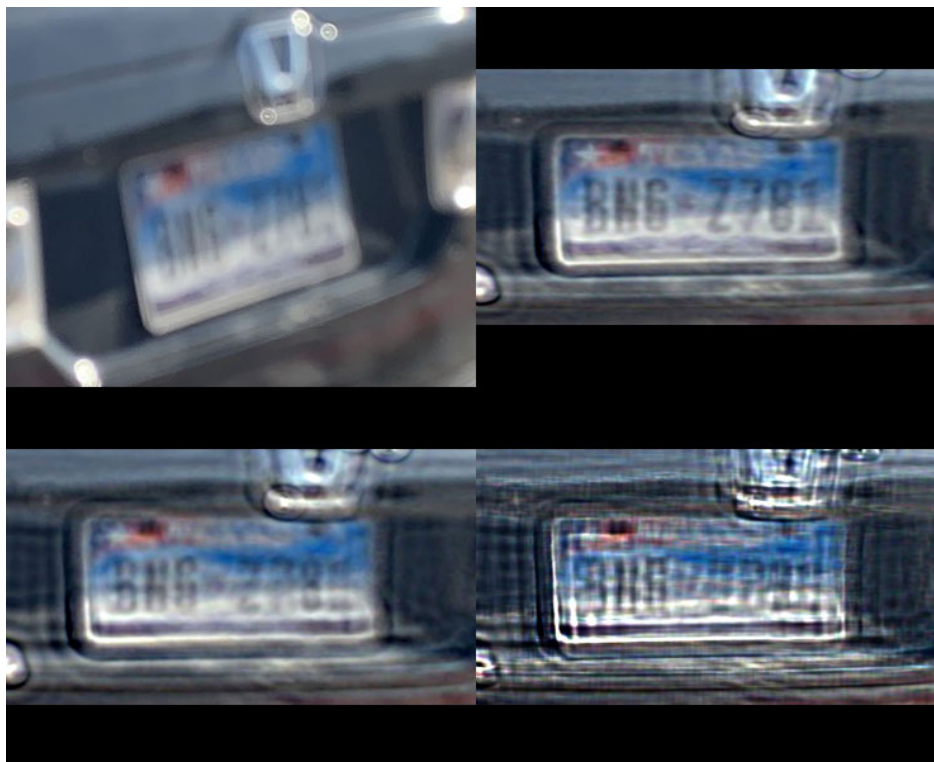
FIGURE 14. Comparison of the three considered restoration workflows on a real image of a license plate affected by a combination of optical blur and mild perspective distortion. Top-left: original image; top-right: proposed workflow (deblur followed by perspective correction); bottom-left: perspective correction followed by deblur; bottom right: perspective correction followed by blind deconvolution.
