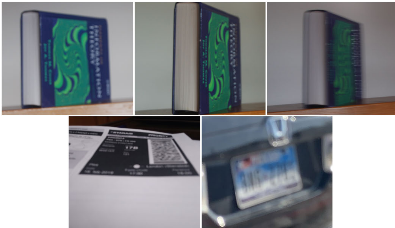
FIGURE 9. Thumbnails of real images considered for restoration. First row: images acquired with a Nikon D50 camera, affected by a combination of optical blur and perspective distortion (first two images) and by motion blur and perspective distortion (third image). Second row, left: image acquired with a Sony Xperia XA1 affected by a combination of optical blur and strong perspective distortion. Second row, right: image acquired with an Apple iPhone XS, affected by a combination of optical blur and mild perspective distortion.
