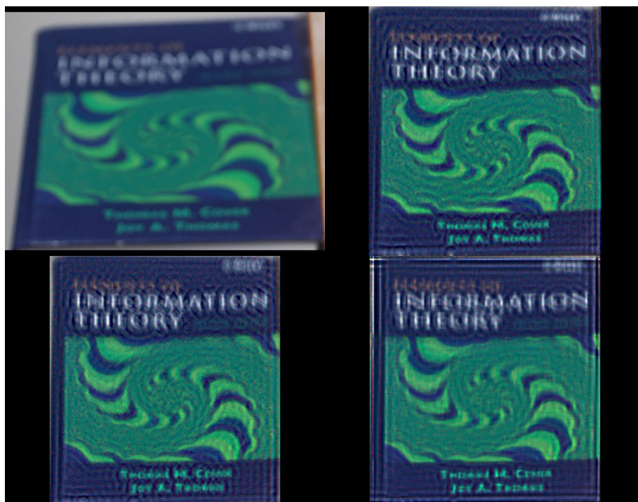
FIGURE 10. Comparison of the three considered restoration workflows on a real image of a book affected by a combination of optical blur and mild perspective distortion. Top-left: original image; top-right: proposed workflow (deblur followed by perspective correction); bottom-left: perspective correction followed by deblur; bottom right: perspective correction followed by blind deconvolution.
