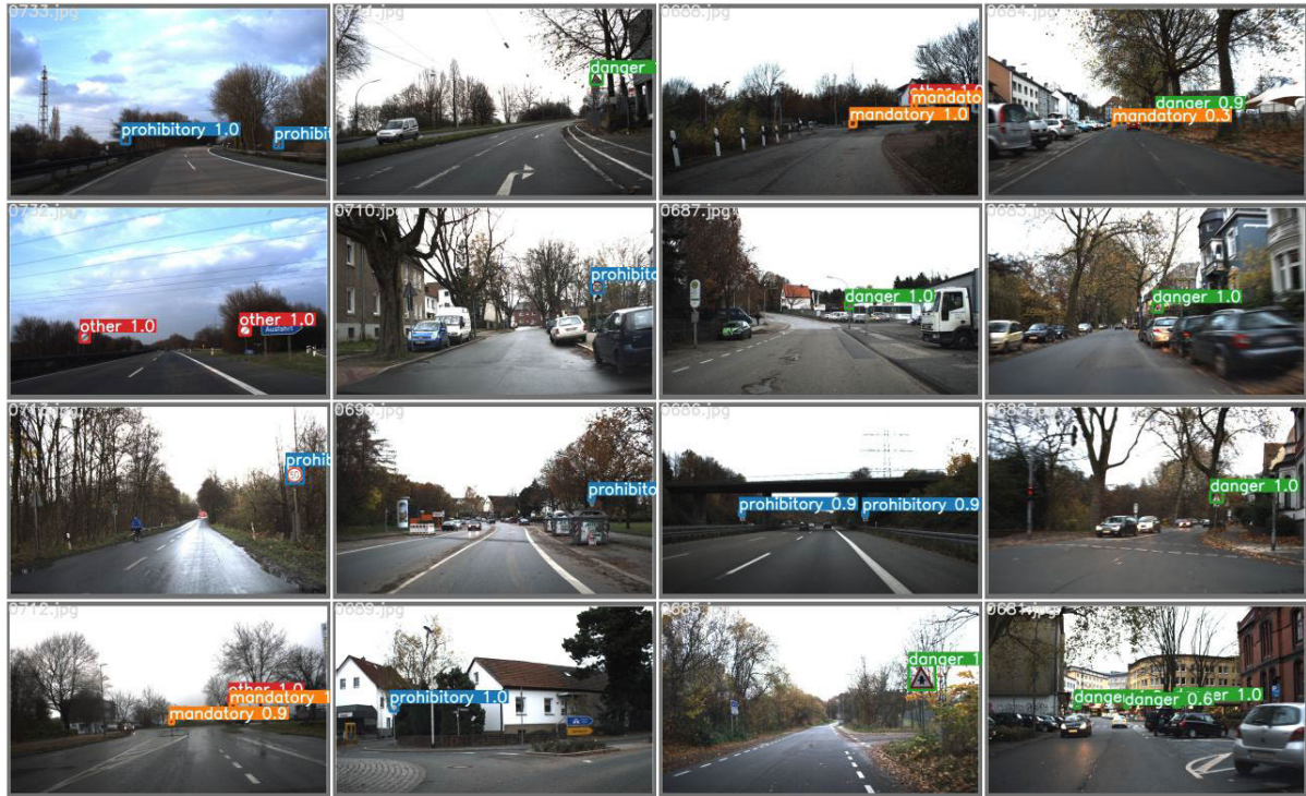
FIGURE 5. Instances of accurate detections in a road environment with small, medium, and large traffic signs belonging to various categories, as generated by the Sign-YOLO framework. All detections shown in these examples are accurate.
