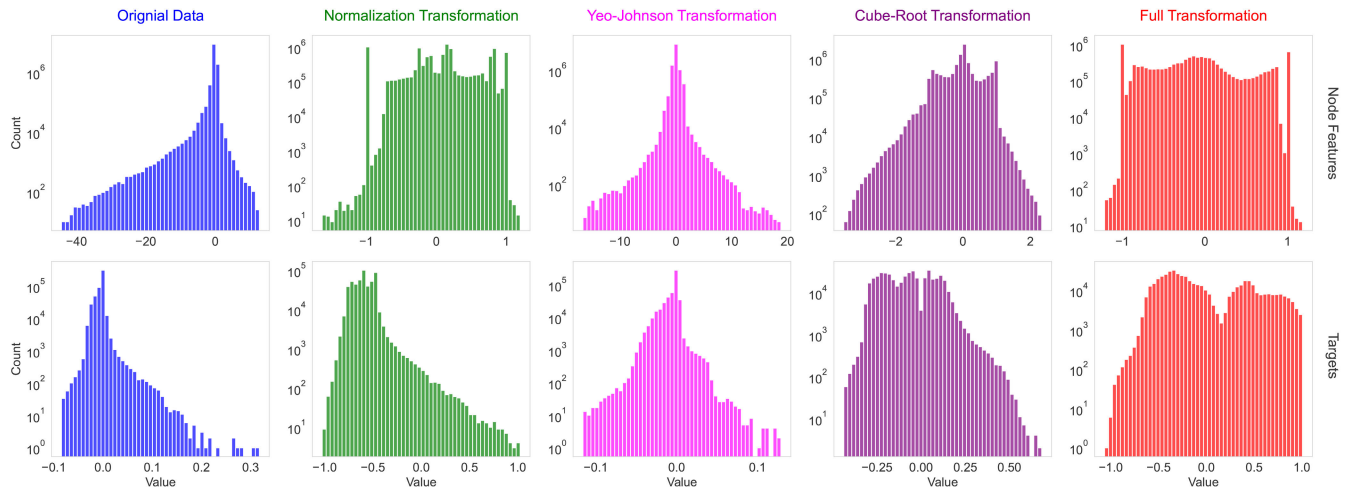
FIGURE 6. Comparison of the effects of various transformations applied individually to each nodal input and output feature dimension, while they are summarized here for visualization. The transformations helped achieve a more standardized normalized distribution when used individually and a more uniform distribution when combined. Such data preparation is critical because it addresses the problem that average evaluation errors are unduly influenced by a majority of simpler nodes rather than a minority of complex nodes, which are typically located in boundary areas with the largest values. These are areas in which the cartilage is exposed to concentrated effects of applied loads and deformations, especially at high loading rates, e.g., at the contact surfaces.
