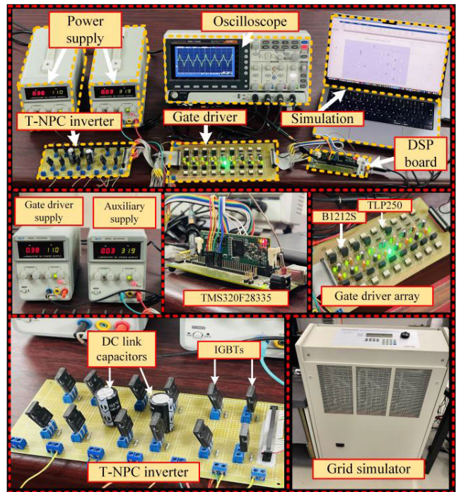
FIGURE 18. A photograph of the laboratory test platform.
