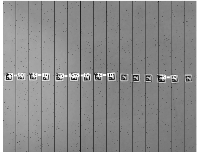
FIGURE 7. Experimental setup for target detection using 4 x 4 cm ArUco markers with added salt-and-pepper noise to simulate a mosaic/noisy background.
