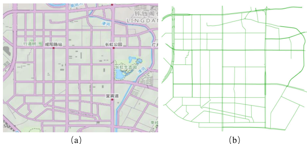
FIGURE 2. The real road network and SUMO road network in the target area. (a) Real road network. (b) SUMO road network.
