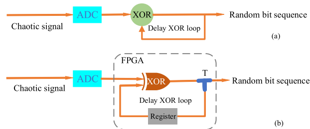
FIGURE 1. Procedure of self-circulating exclusive-or (XOR) method. (a) the profile of self-circulating XOR, and (b) the schematic of self-circulating XOR implemented in a field programmable gate array. ADC: analog-to-digital converter. XOR: exclusive-or. T: T-type connector. FPGA: field programmable gate array.
