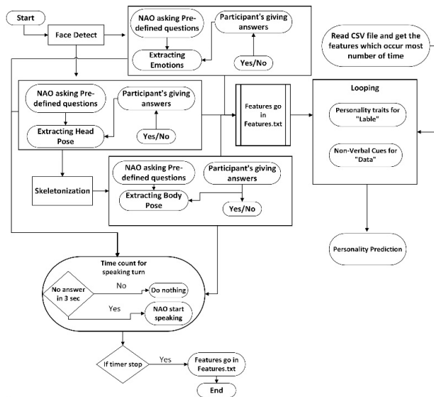
FIGURE 2. System flowchart for complete architecture explaining personality prediction based on Human-Robot Interaction (HRI).
