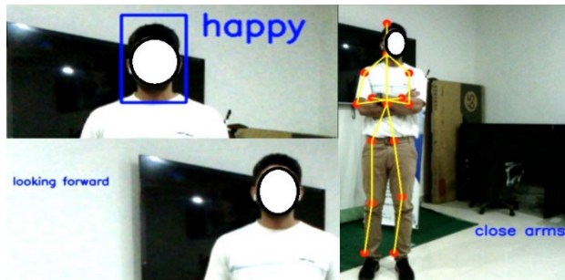
FIGURE 6. Labelling of different modules using NAO camera during a human-robot interaction.
