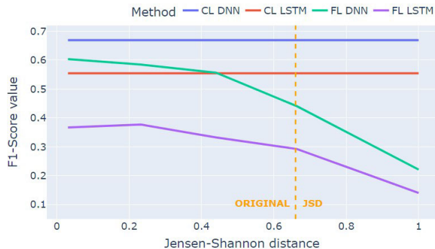
FIGURE 3. F1-Score of the DNN and LSTM models on the Physionet dataset for CL, and the Physionet dataset partitioned for four clients to achieve different label skewness as measured based on JSD, for FL using FedAvg.
