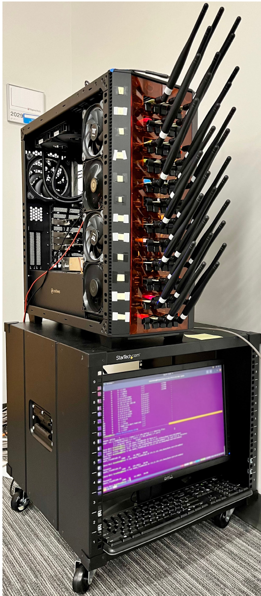
FIGURE 5. The transmit-side hardware setup of the transmitter host and attached YARD Stick One radios on the front USB hub array.
