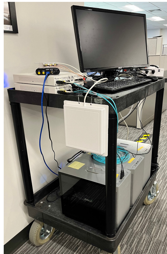
FIGURE 4. The receive-side hardware setup with collection nodes and their attached radios. The collection nodes are located on the lower shelf while the radios are placed on the top of the cart.
