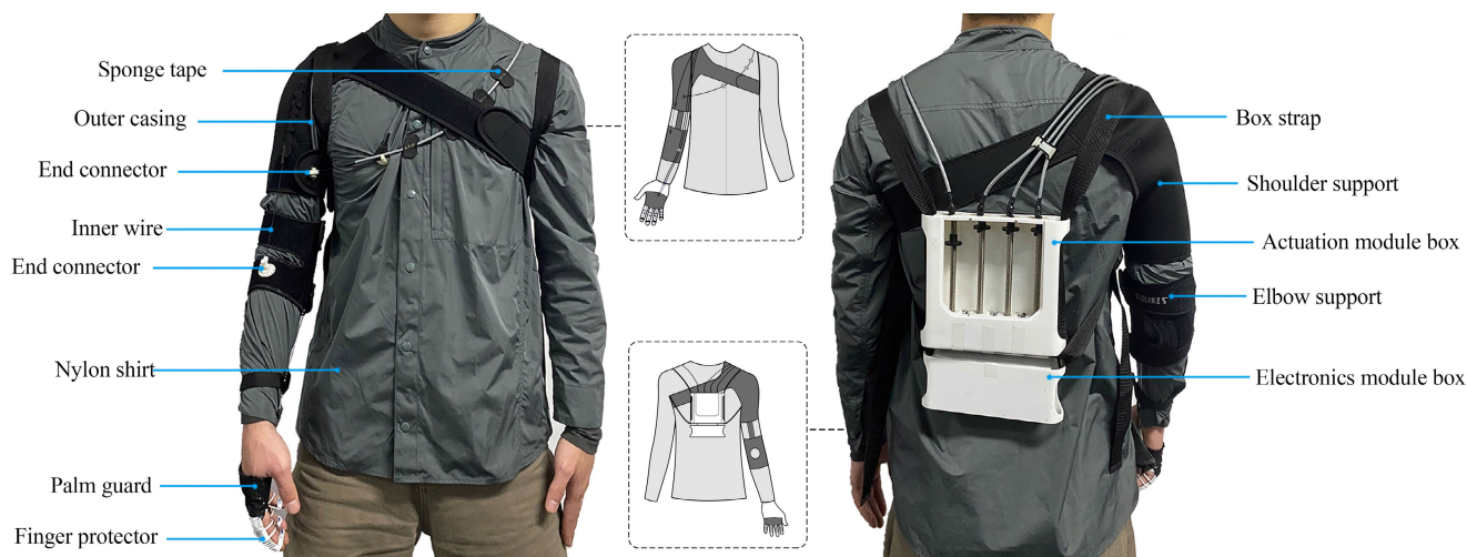
FIGURE 1. Hardware structure.
