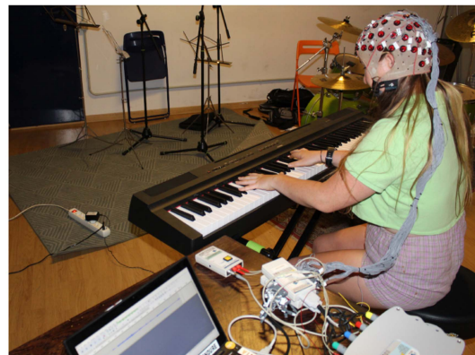
Fig. 1. Data acquisition system setup: Biosignal electrodes (EEG and ECG) are connected to two g.USBAMP biosignal amplifiers via two separate g.GAMMAbox's with a laptop recording the amplified data via USB in Simulink; acoustic signals were recorded on the same computer using a soundcard.
