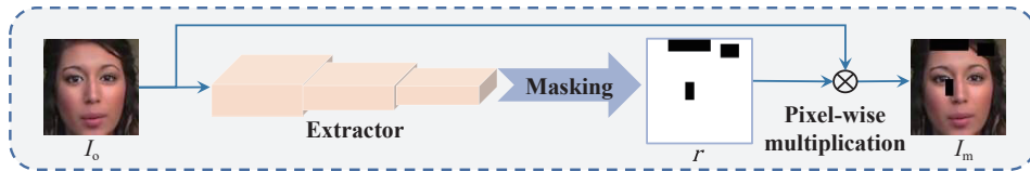
Fig. 2 Forged trace masking module (FTMM) uses an extractor to calculate the gradients of the original image for masking the highly suspected regions.
