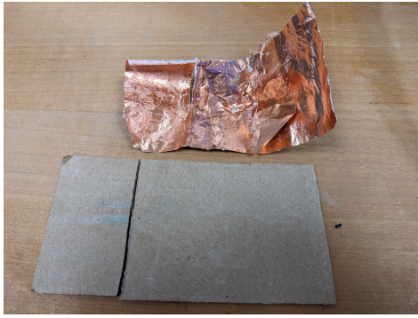
Fig. 31. Separated materials of the harmonic crack sensor for recycling: copper foil, cardboard, and surface-mounted components.
