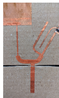
Fig. 30. Harmonic tag for crack sensing. (a) Schematic of the via-less frequency doubler. (b) Photograph of the proof-of-concept prototype on cardboard. (c) Photograph of the measurement setup. (d) Detail of the stub after break. (e) Received second harmonic power.
