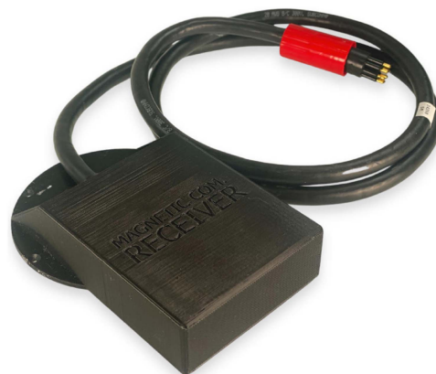
Fig. 9. UMWC receiver based on four high-sensitivity AMR broadband sensors. The signal from each sensor is amplified, spatially averaged and demodulated on board. The receiver circuitry is pressure-neutral encapsulated.
