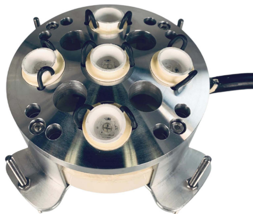
Fig. 10. Transmitter for UOWC comprising five high-power royal blue LEDs. The LED drivers are potted with thermally conductive resin and placed below the diodes which are arranged on a CNC-milled mount. This design provides optimal cooling and is space- and weight-saving.
