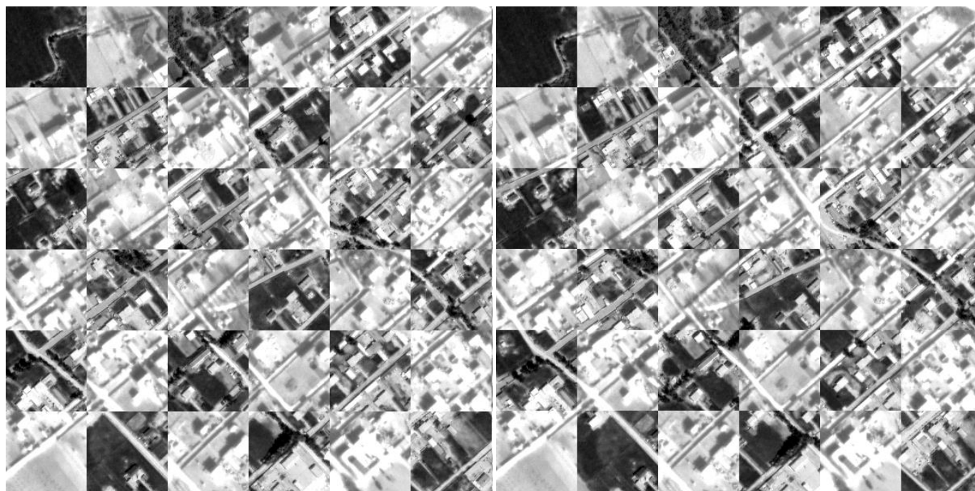
Fig. 13. Comparison of checkerboard patterns of CCD3 image products in G01 before and after S01 parameters processing
