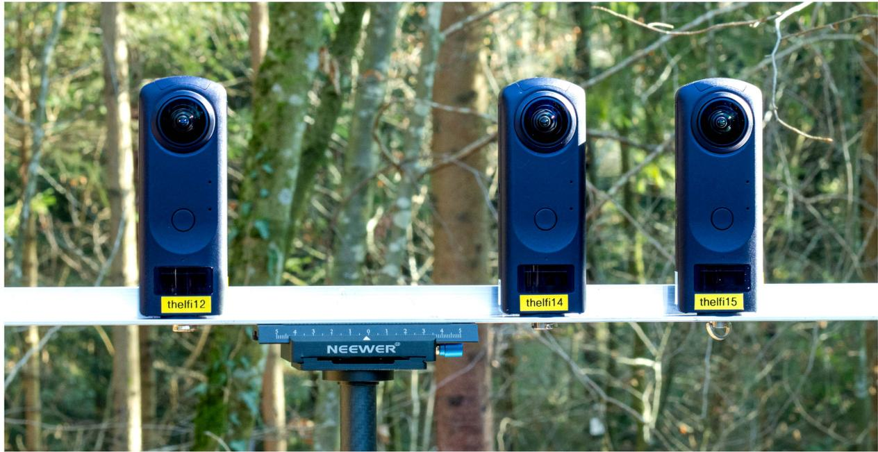
Fig. 2. Stereo video system used in this study targeted two dual-lens fish-eye Ricoh Theta Z1 cameras with a known baseline (distance between the camera sensors). To foster comparability, we used three spherical cameras arranged on a hand-held gimbal to simultaneously capture stereo videos with three baselines, namely, 20, 40, and 60 cm.
