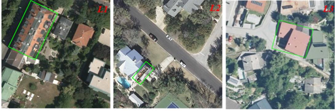
Fig. 2. (L1) Heterogeneity at the top of the building, (L2) clutter covering the top of the building, and (L3) shadow blocking at the top of the building.
