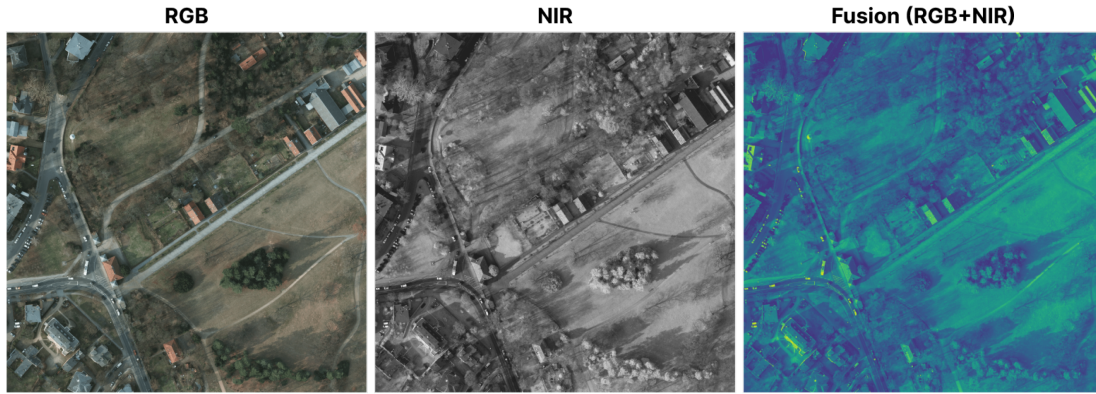
Fig. 19. Graphical visualization of the fusion of RGB channels with NIR using averaging on an image from the Potsdam dataset.
