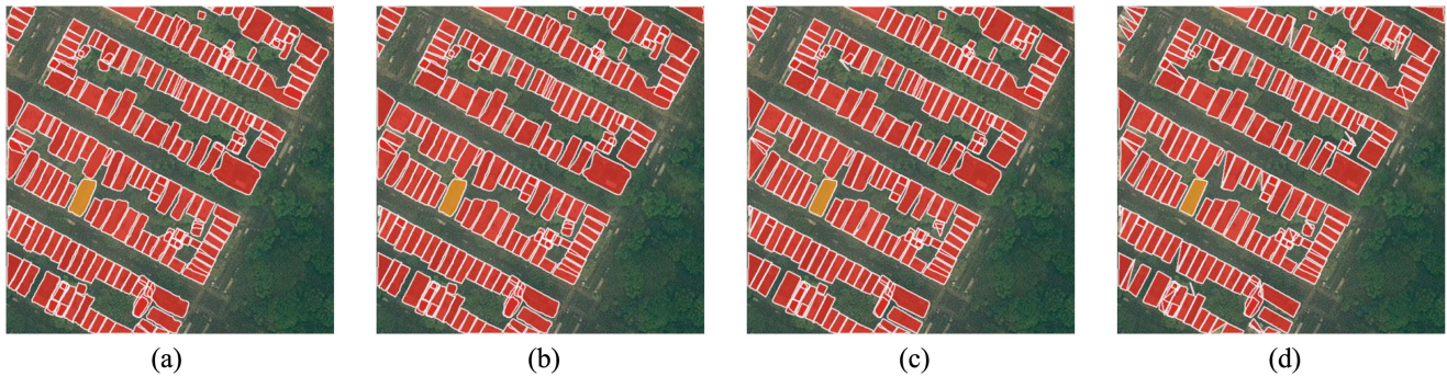
Fig. 11. Visualized results under different vertex reduction threshold S_{\text{cnr}} . (a) S_{\text{cnr}} = 0.05 . (b) S_{\text{cnr}} = 0.1 . (c) S_{\text{cnr}} = 0.2 . (d) S_{\text{cnr}} = 0.3 .
