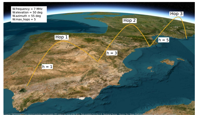
Fig. 5. Simulation of a ray traced from Seville (Spain) in the direction to Barcelona with an elevation of 50 ^{\circ} to illustrate the concept of “hops.” Each time a new hop is started, the internal variable h is increased by 2.
