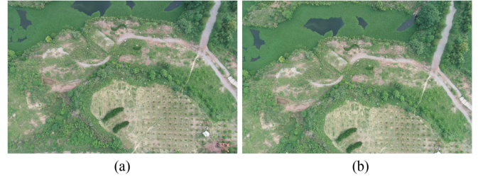
Fig. 5. Sample pair of images. This pair of images shows that due to the absence of prominent features, the prediction of height is not very accurate. (a) Left image. (b) Right image.
