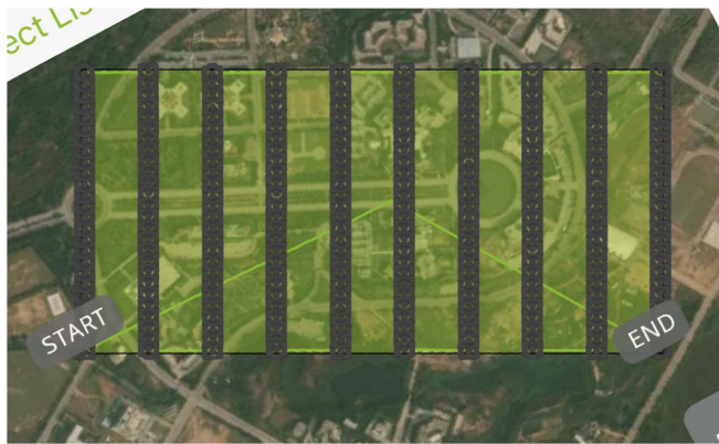
Fig. 3. Pix4dcapture mobile app [36] is used to capture the dataset. This app has the option to enter the complete flight path along with start and end points as well as the percentage of overlapping required among consecutive images. The figure shows the start, end, and the complete path of drone flight for capturing the dataset. The black lines (drone flight path) indicate the position of images taken during flight. The image pair at the end of each path and the start of the new path was ignored as they have little overlapping.
